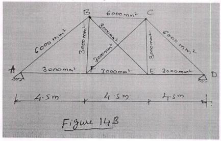
15. A). Derive the member stiffness matrix for plane truss member.
