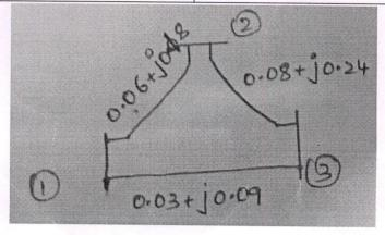
11. B). For the 3-bus system shown in the figure, Obtain the  $Z_{bus}$
