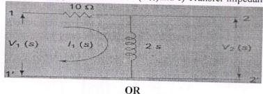
13. B). Draw the pole zero diagram for the given network function I(s) and hence obtain i(t).
