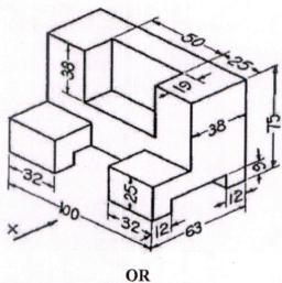
15. B). Draw the isometric projection as per given figure below.
