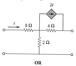
13. B). Derive the ABCD parameters in terms of Z parameters.
