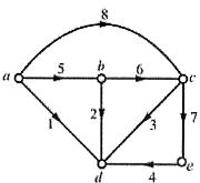
ii) Draw the graph of the circuit shown below and select a suitable tree to write tie-set matrix.
